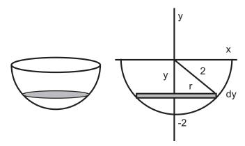
I've drawn the tank in cross-section as a semicircle of radius 2 extending from y = -2 to y = 0. Divide the volume of water up into circular slices. The radius of a slice is  $r = \sqrt{4 - y^2}$ , so the volume of a slice is  $dV = \pi r^2 dy = \pi (4 - y^2) dy$ . The weight of a slice is  $62.4\pi (4 - y^2) dy$ , where I'm using 62.4 pounds per cubic foot as the density of water.
